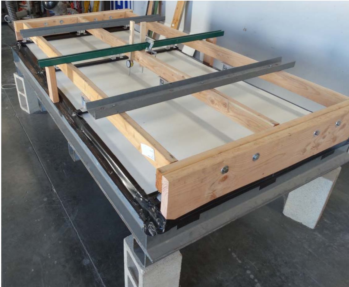
Photograph No.3 ES-400 negative load test setup.
