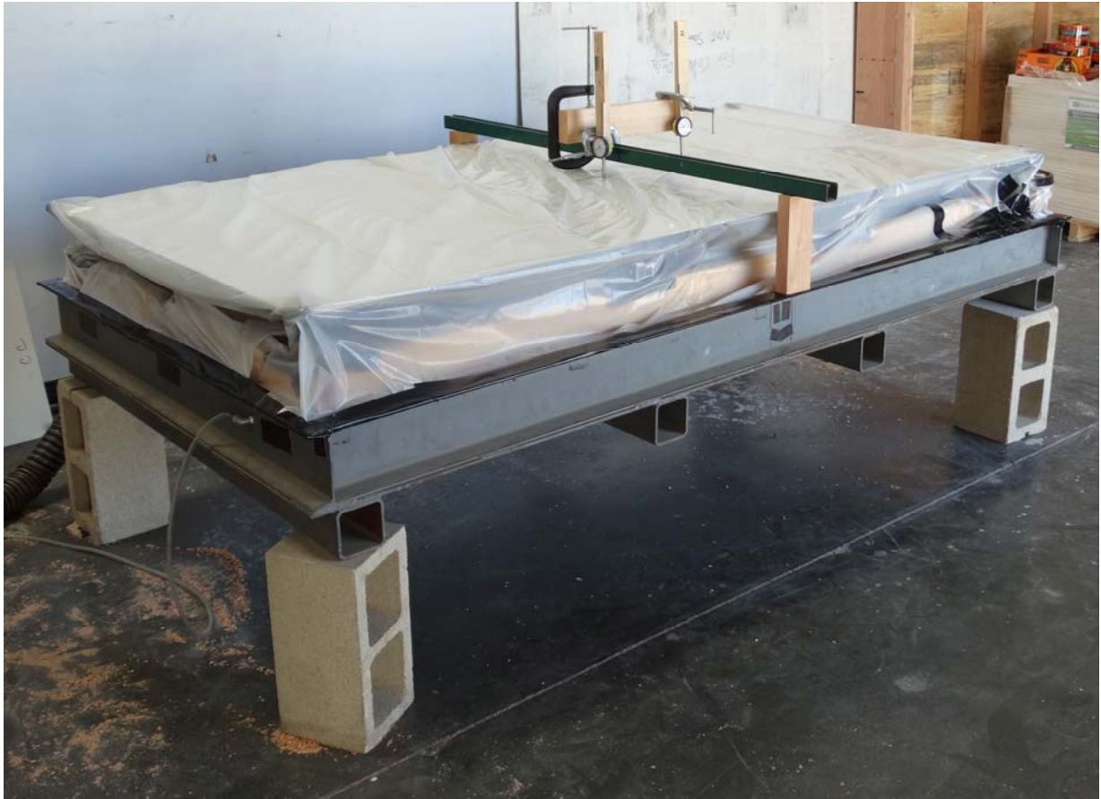
Photograph No.4 ES-400 positive load test setup.
