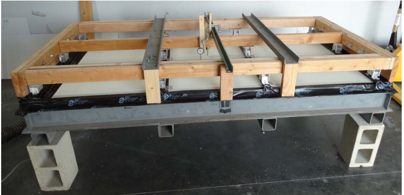
Photograph No.1 ES-500 negative load test setup.
