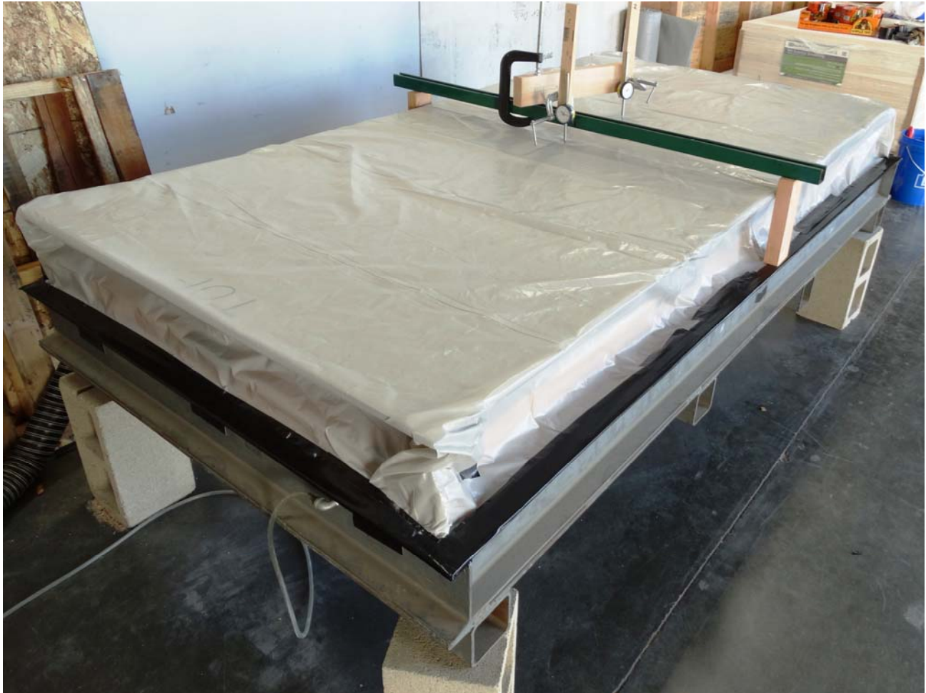
Photograph No.2 ES-500 positive load test setup.
