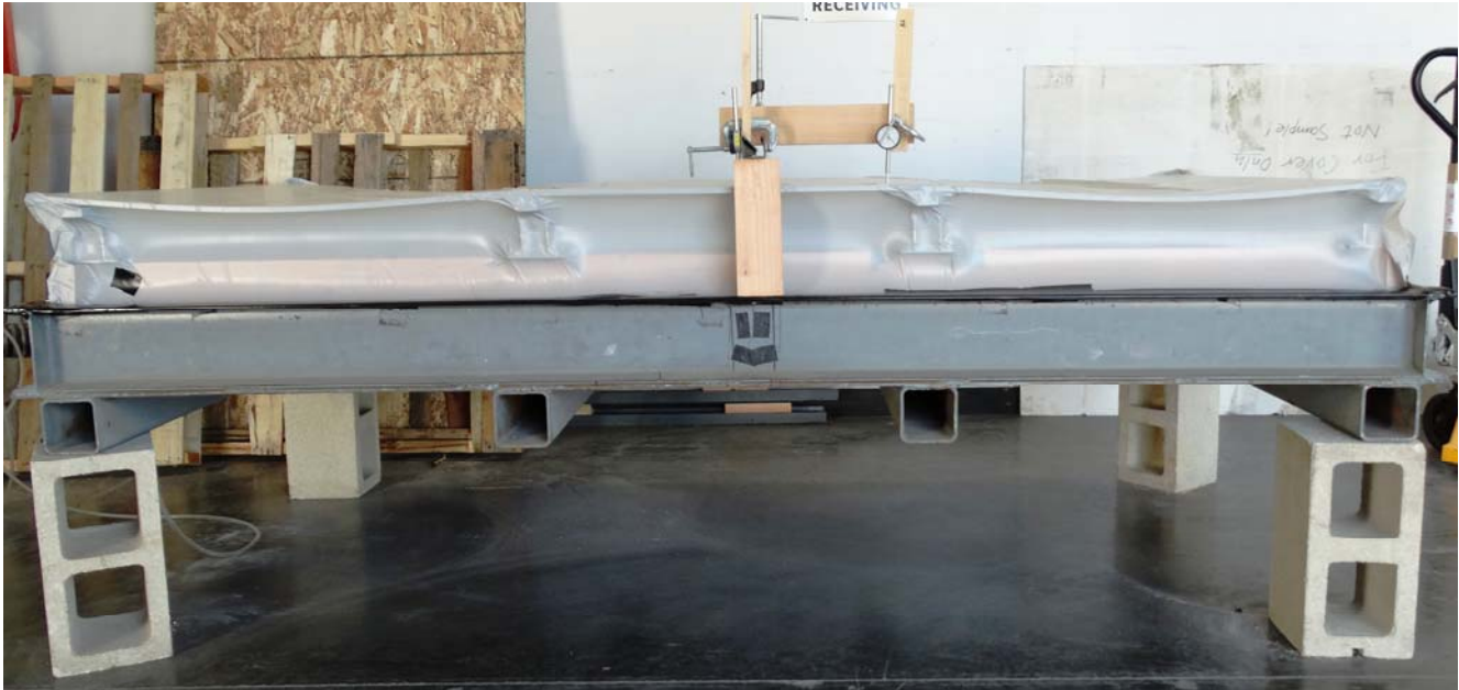
Photograph No.5 ES-500 positive load test
