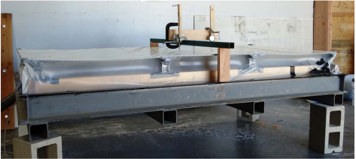
Photograph No.7 ES-400 positive load test
